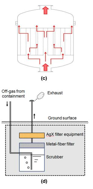
Fig. 1 Diagram of AgX filter unit and its application. (a) Top view; (b) Front view and dimensions; (c) Flow path; (d) Application to WET-system.
